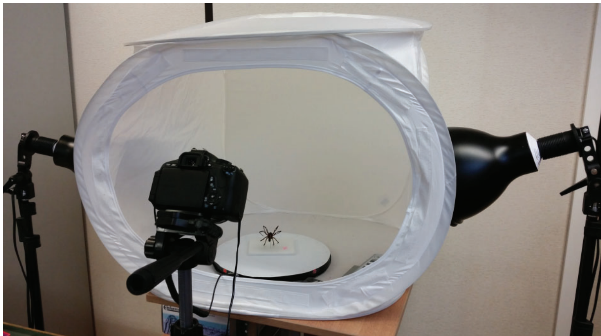
Fig. 3.1. Photogrammetry set-up with a specimen on a manual turntable, a Canon DSLR on a tripod, 2 studio lights and a light tent.
